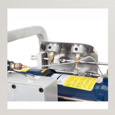
Slightly bend up reset button tube toward sky without breaking, and carefully slide motor assembly away from the air condenser.
