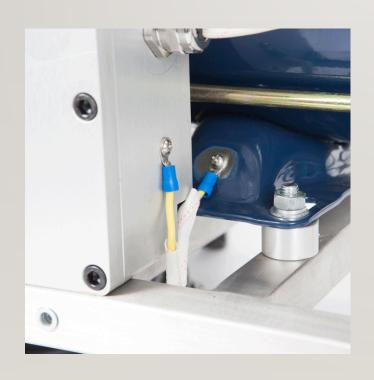
Remove motor chassis bolts using the 14 mm Wrenches and disconnect ground wire (usually a yellow wire with white jacket) from the pump power box.
